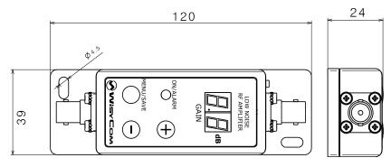
BAA is wideband antenna booster especially designed to allow using long cables with broadband wireless receiver system working in 470-960 MHz thanks to a very high OIP3 of 40 dBm.
