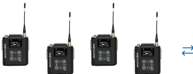
Remote control with the MRK16 as a bridge allows management of the MTP60 over hundreds of meters
