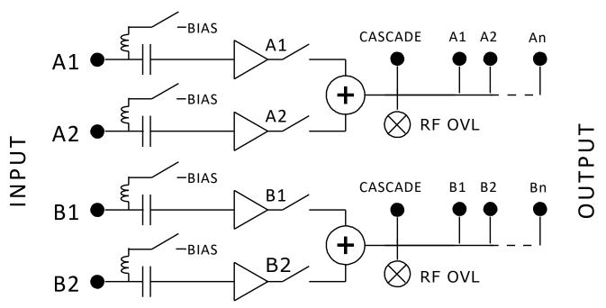
It provides antenna bias & diagnostic check and integrates the **Wisycom Remote Antenna Protocol**: using the same coaxial cable it creates a network to monitor and control remotely boosters (BFA) or antennas (LFA). Thanks to the ethernet interface all of these functionalities can be supported on the PC using the Wisycom Wireless Manager program.
