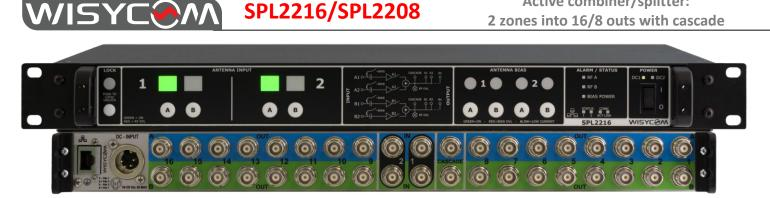
SPL2216/SPL2208 is an **active** combiner/splitter: **2 x 2 (diversity) input** are combined and then distributed in **16 x 2 diversity outputs** (for SPL2216) or **8 x 2 diversity outputs** (for SPL2208). It allows a basic matrix-selection between 2 diversity areas: *each input feed can be activated with a button on the front panel.*
