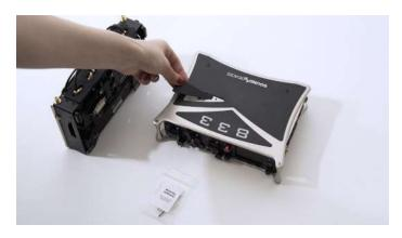
STEP 2 Using a #4 Phillips Screwdriver, remove the two black phillips screws from the 833/888 top panel as shown in the image below. Keep these screws in a safe place as they need to be re-installed if the SL-2 is removed from the 833/888.
