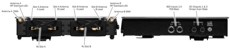
**ANTENNA A & B SMA CONNECTORS** Connects antenna to the SL-2. Both SMA antenna connectors can provide 12 V bias power up to 500 mA via a menu option. RF frequency range covers 470 - 1525 MHz. RF Filtering is available in the menus.
