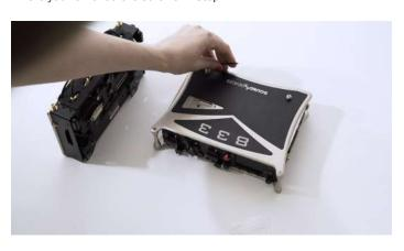
STEP 4 Align the SL-2's bottom panel hooks with the Rear Keyhole Pegs on the 833/888. The SL-2 should be tilted with the front panel slightly higher than the rear. Take care not to bump the SL-2 expansion connector against the 833/888 top panel. Once the SL-2's Bottom Panel hooks and Rear Keyhole Peg's machined grooves are aligned, slide the SL-2 towards the front panel.
