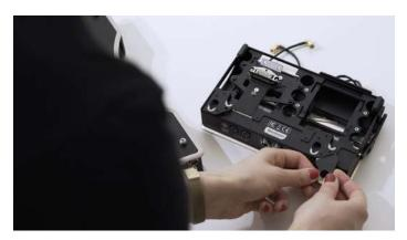
**STEP 6** Align the SL-2 Rear Bracket and the Rear Keyhole Peg on the Scorpio. The SL-2 should be tilted with the front panel slightly higher than the rear. Take care not to bump the SL-2 Expansion Connector against the Scorpio top panel. Lower the rear of the SL-2 Rear Bracket onto the Rear Keyhole Peg on the Scorpio. Once the SL-2 Rear Bracket and Rear Keyhole Peg's machined grooves are aligned, slide the SL-2 towards the front panel.
