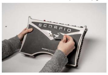
**STEP 2** Using a #4 Phillips Screwdriver, remove the black phillips screw from the Scorpio top panel as shown in the image below. Keep these screws in a safe place as they need to be re-installed if the SL-2 is removed from the Scorpio.
