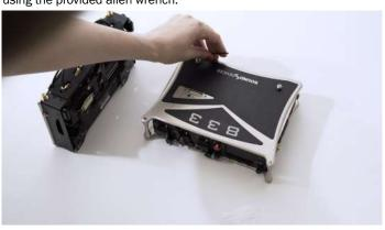
**STEP 5** Replace the originally provided rear black screws near the Sound Devices logo using #4 Phillips head screwdriver.
