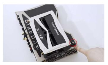
**STEP 7** Make sure that the SL-2 Expansion Connector mates with the Scorpio Expansion Port. Then gently press down on the SL-2 to fully seat the pins of the connector.
