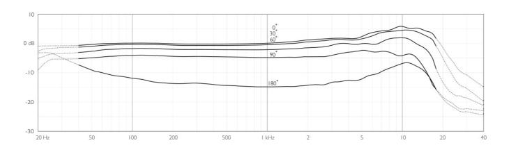
Typical on and off-axis response of a DPA 4055 Kick Drum Microphone measured at 20 cm (7.9 in)
