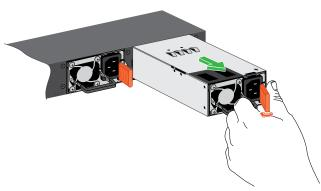
3. Insert the replacement APS into the power module bay, and gently push the APS into the bay until the latch locks.
