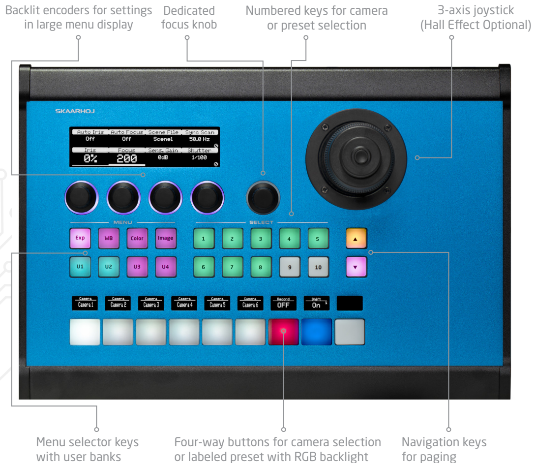
Hardware Option: Hall Effect joystick for increased precision and ergonomics of operation
